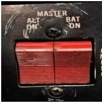
Figura 3. Interruptor principal (master switch)
