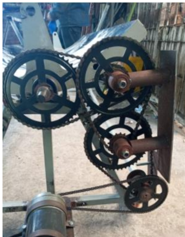
Fig 2. Solar tracking mechanism
