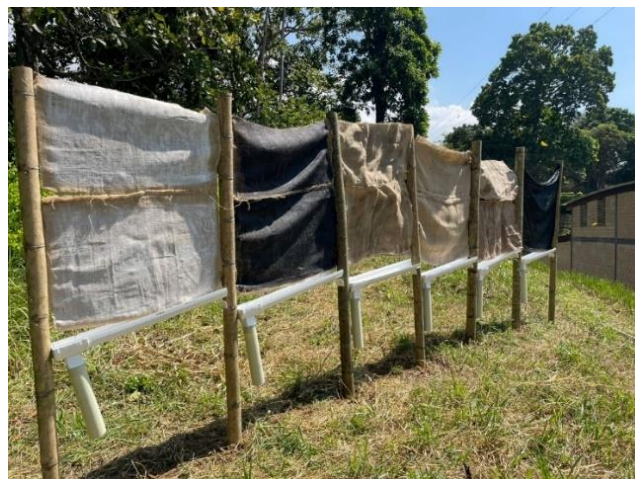
Fig. 6. Fog catchers manufactured and installed
