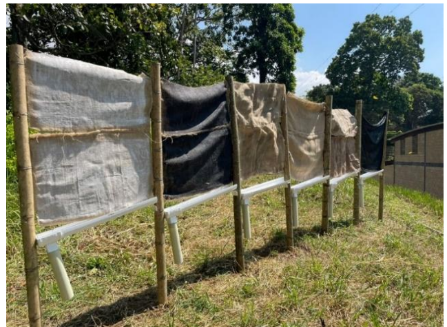
Fig. 6. Fog catchers manufactured and installed
