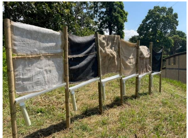
Fig. 6. Fog catchers manufactured and installed
