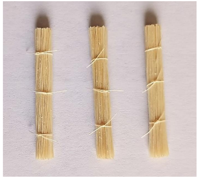
Fig. 5. Groups of 200 fique fibers for density measurement using Archimedes' principle.
