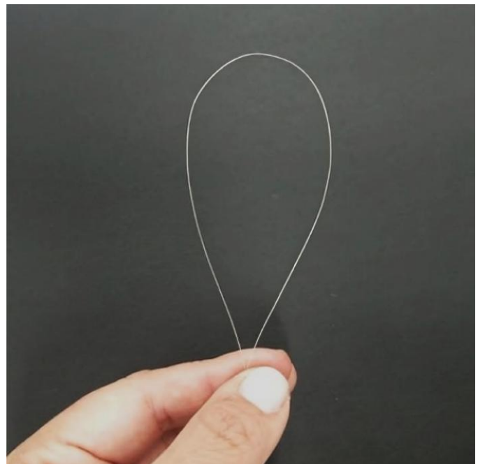
Fig. 3. Loop test to verify the absence of defects along the technical fiber.
