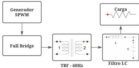
Fig. 5. Block diagram of second prototype DC/AC converter. Source: own
